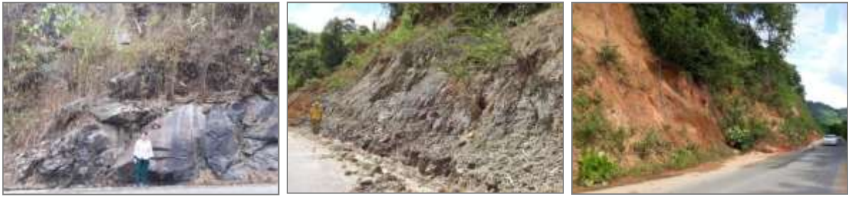
Figure 3 Type-A Profile: (1) fresh rock (N 25° 24' 32.2" and E 97° 58' 01.5"), (2) decomposed granitoid (N 25° 22' 25.2" and E 97° 44' 57.3"), and (3) residual soil (N 25° 23' 46.2" and E 97° 38' 40.5").
